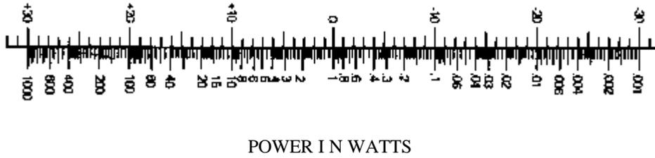
Figure 2-1. Nomograph for Determining Power Ratios Directly in dB
