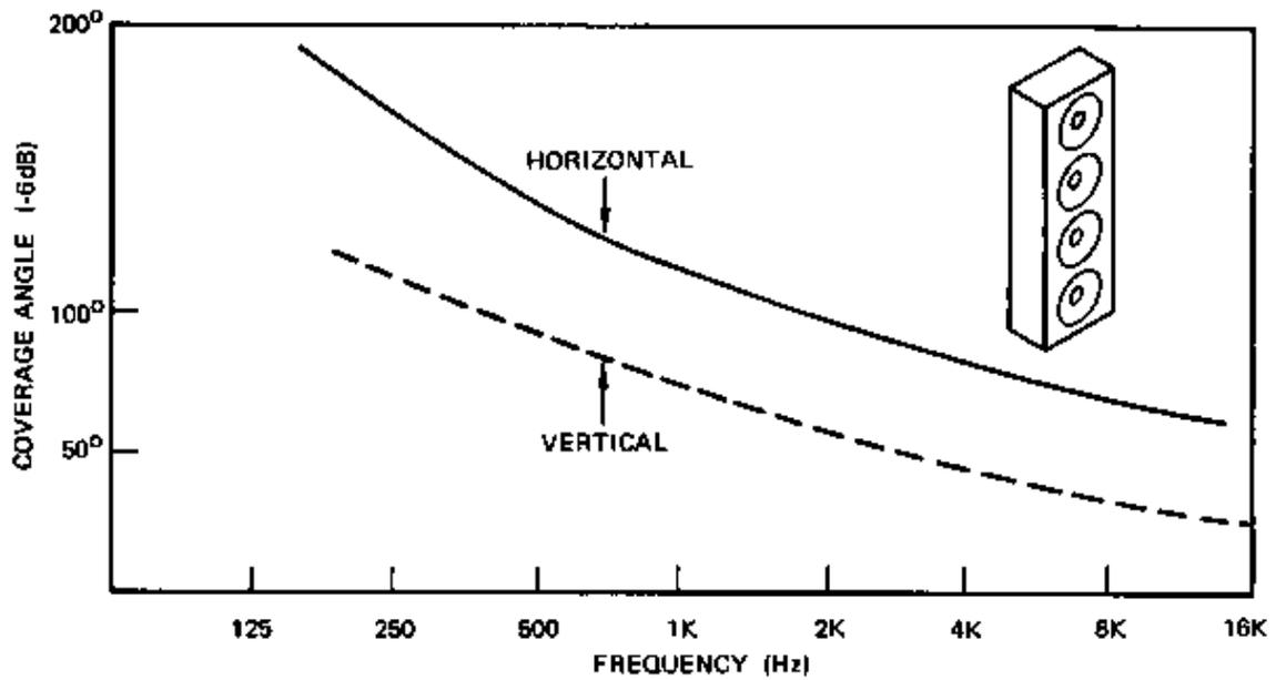
Figure 7-12. Directivity Characteristics of a Sound Column
