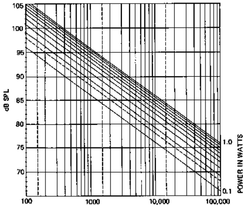
Figure 5-21. Steady-State Reverberant Field SPL vs. Acoustic Power and Room Constant
