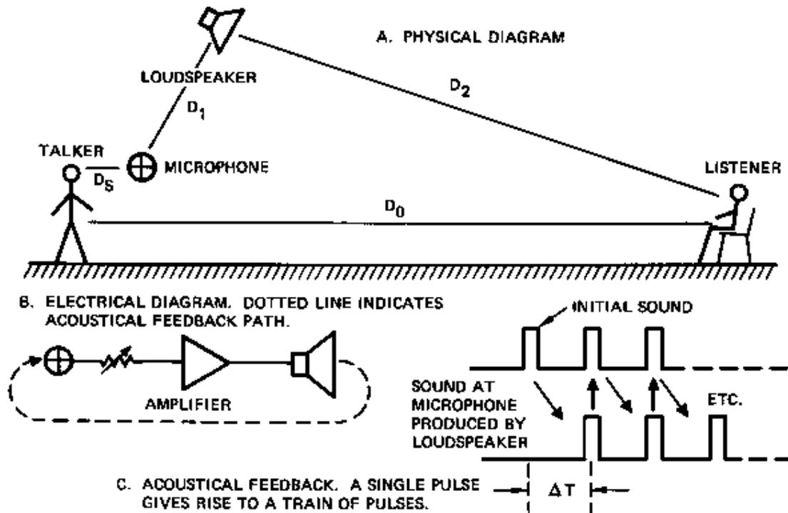
Figure 4-1. A Simple Outdoor Reinforcement System
