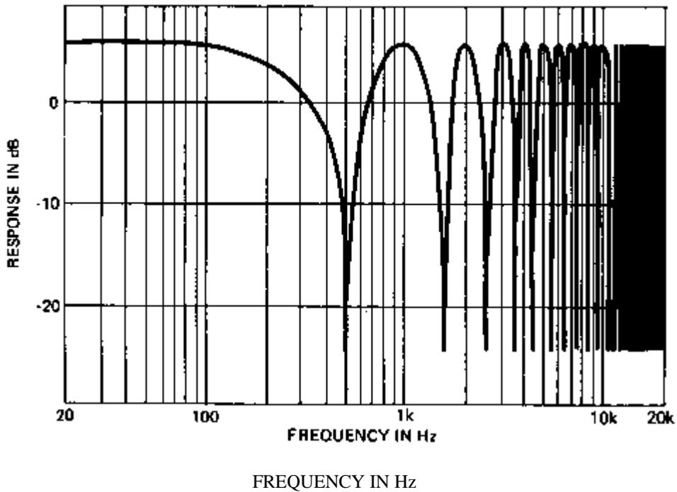
FREQUENCY RESPONSE OF TWO WIDE-RANGE PROGRAM CHANNELS COMBINED WITH ONE MILLISECOND DELAY BETWEEN CHANNELS. SAME PROGRAM SIGNAL FED TO BOTH, EXCEPT THAT AMPLITUDES DIFFER BY 0.5 dB.
