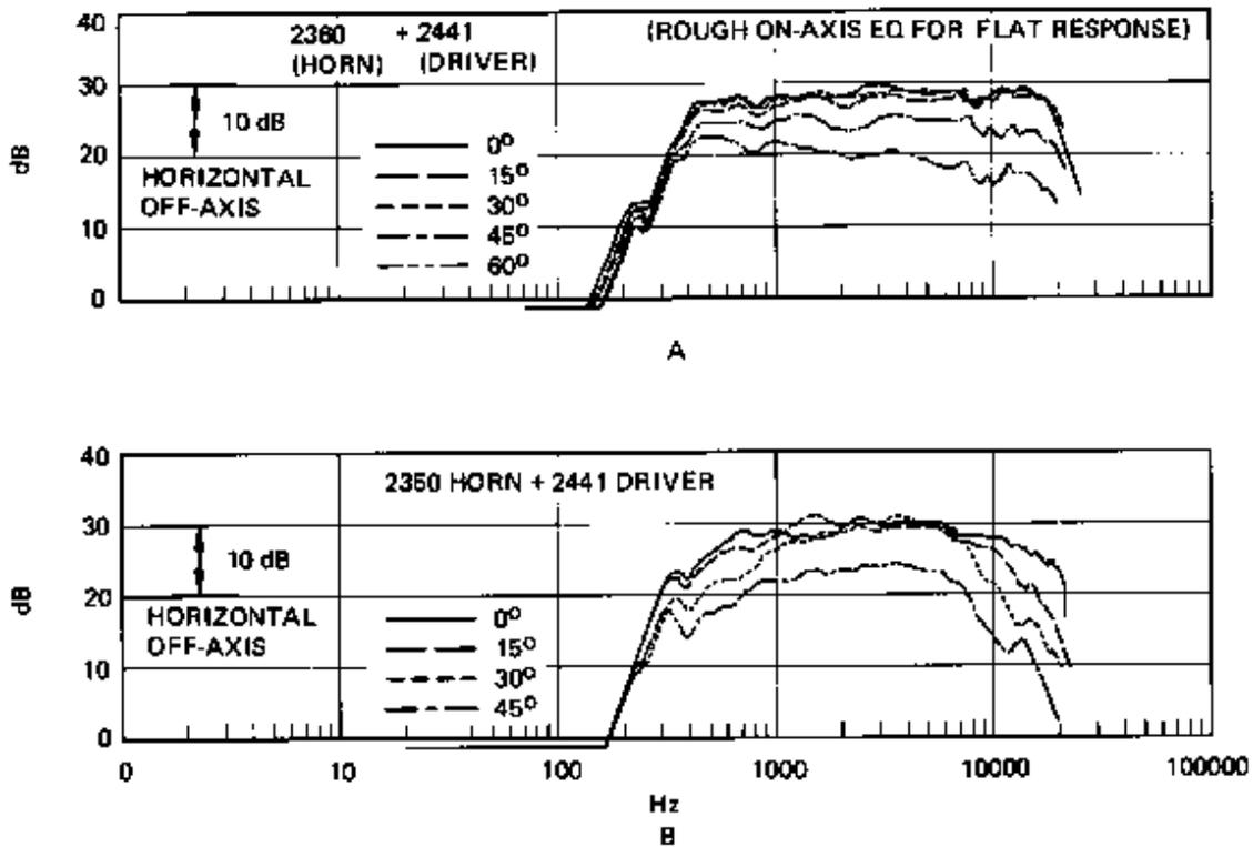
Figure 36. Families of Off-Axis Frequency Response Curves
