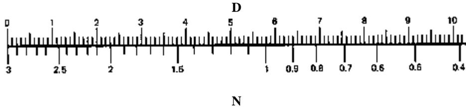
Figure 2-7. Nomograph for Adding Levels Expressed in dB. Summing Sound Level Output of Two Sound Sources Where D is Their Output Difference in dB, N, is Added to the Higher Level to Derive Total Level
