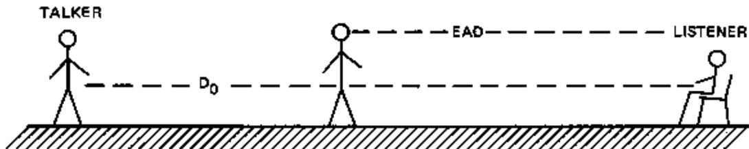
Figure 4-6. Concept of Effective Acoustical Distance (EAD)
