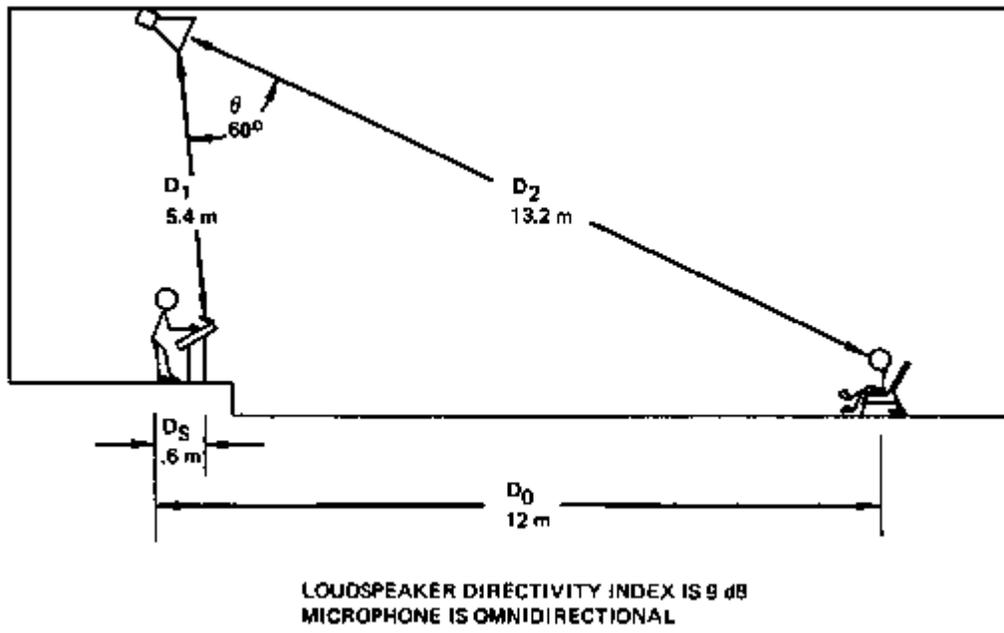
Figure 6-5. Sound System in a Medium-Size Room, Gain Calculations
