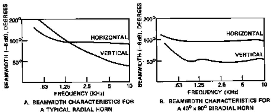
Figure 343. Increasing DI through Narrowing Vertical Beamwidth
