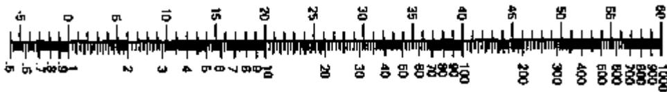
Figure 2-6. Nomograph for Determining Inverse Square Losses
