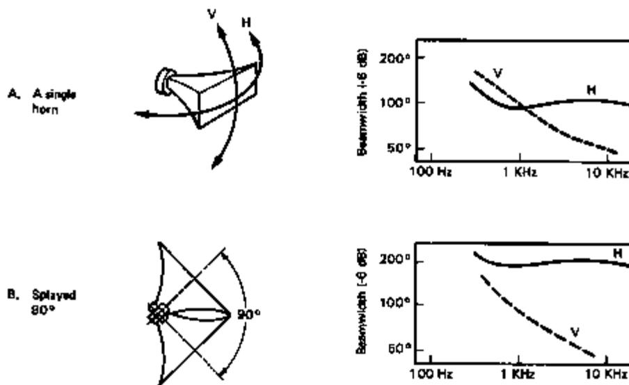
Figure 3-12. Horn Splaying for Wider Coverage
