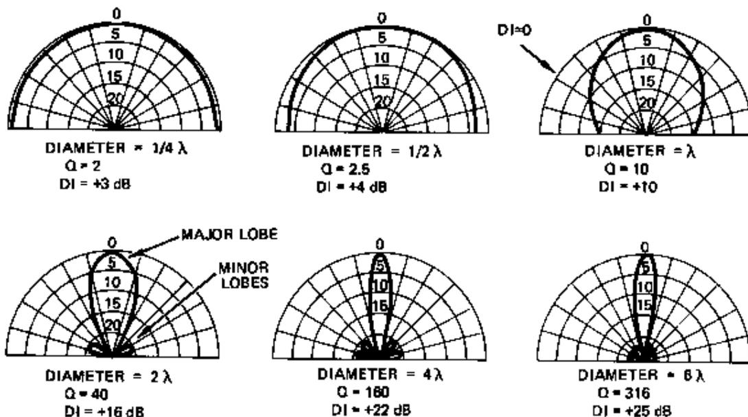
Figure 3-6. Directional Characteristics of a Circular-Piston Source Mounted in an Infinite Baffle as a Function of Diameter and  $\lambda$ .
