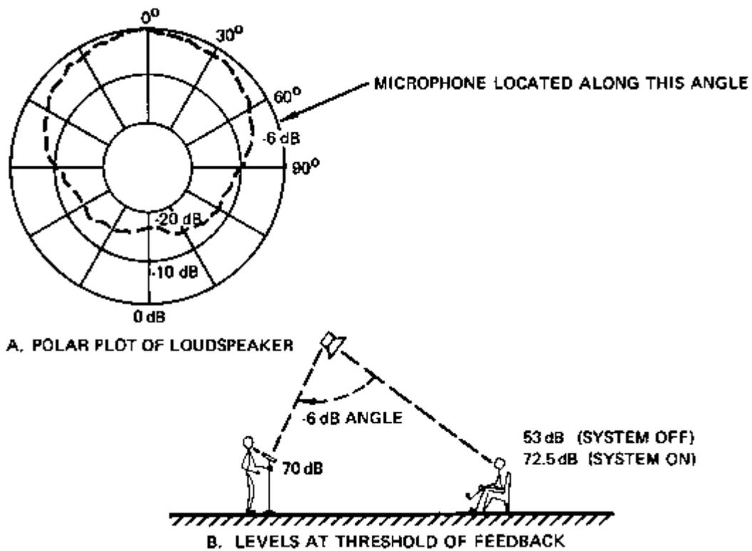
Figure 4-4. System Gain Calculations, Directional Loudspeaker
