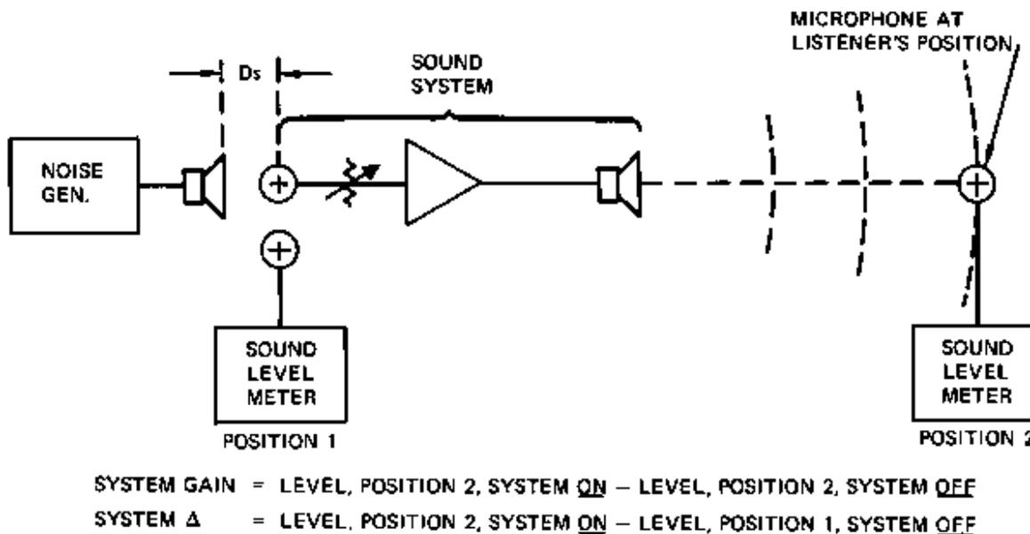
Figure 6-11. Measurement of Sound System Gain and Delta ( )
