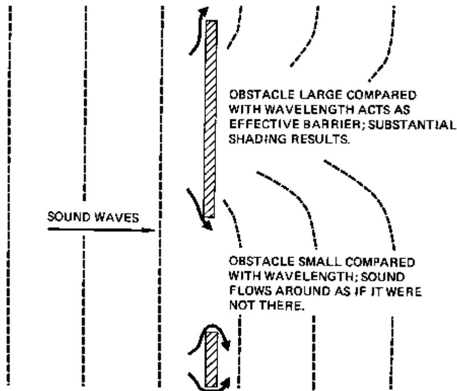
Figure 1-7. Diffraction of Sound Around Obstacles
