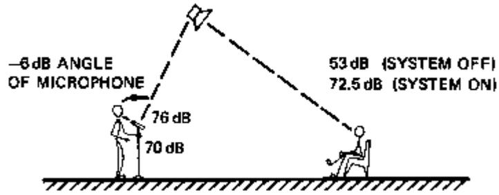
B. LEVELS AT THRESHOLD OF FEEDBACK
