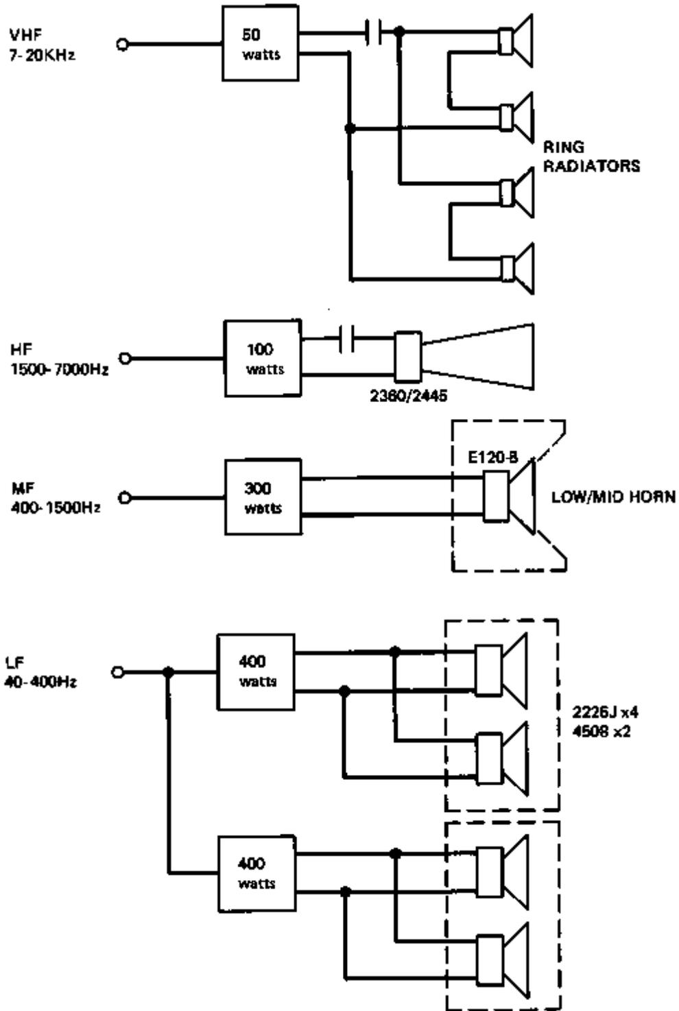
Figure 7-20. A Four-way System of High Output Capability
