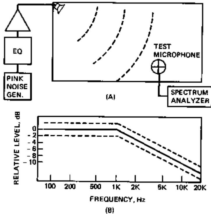
Figure 6-17. Sound System Equalization Procedure
