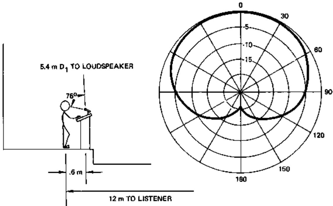
Figure 6-7. Characteristics of a Cardioid Microphone
