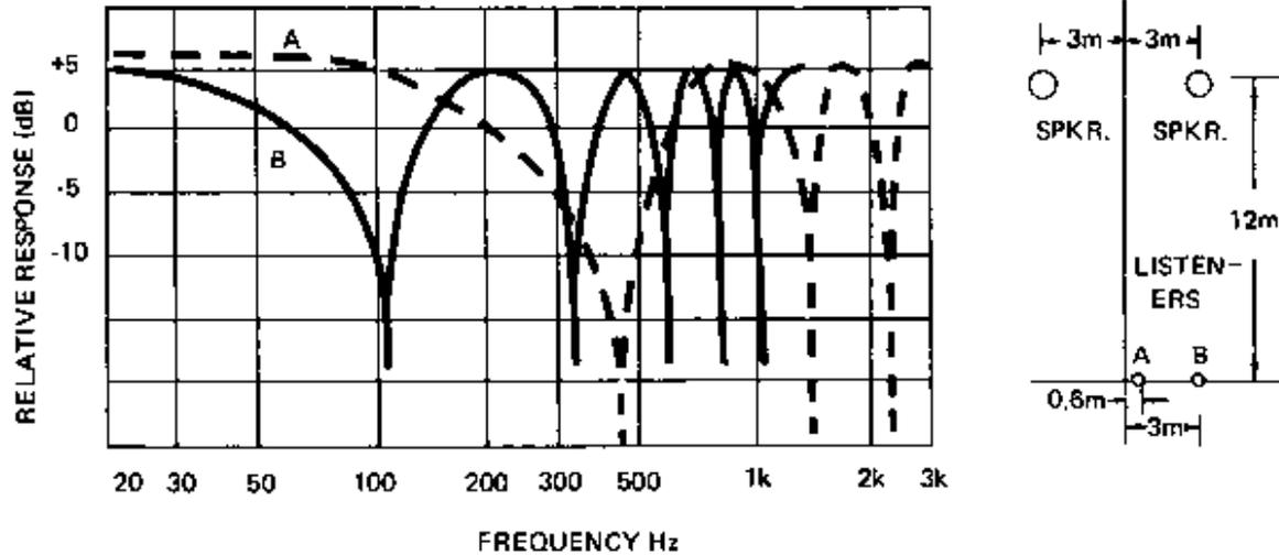
Interference Effects from Two Separated Loudspeakers Producing Coherent Signals
