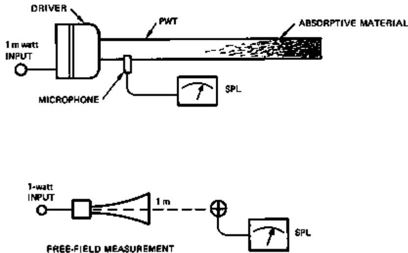
Figure 3-10. PWT Method for Measuring Directivity
