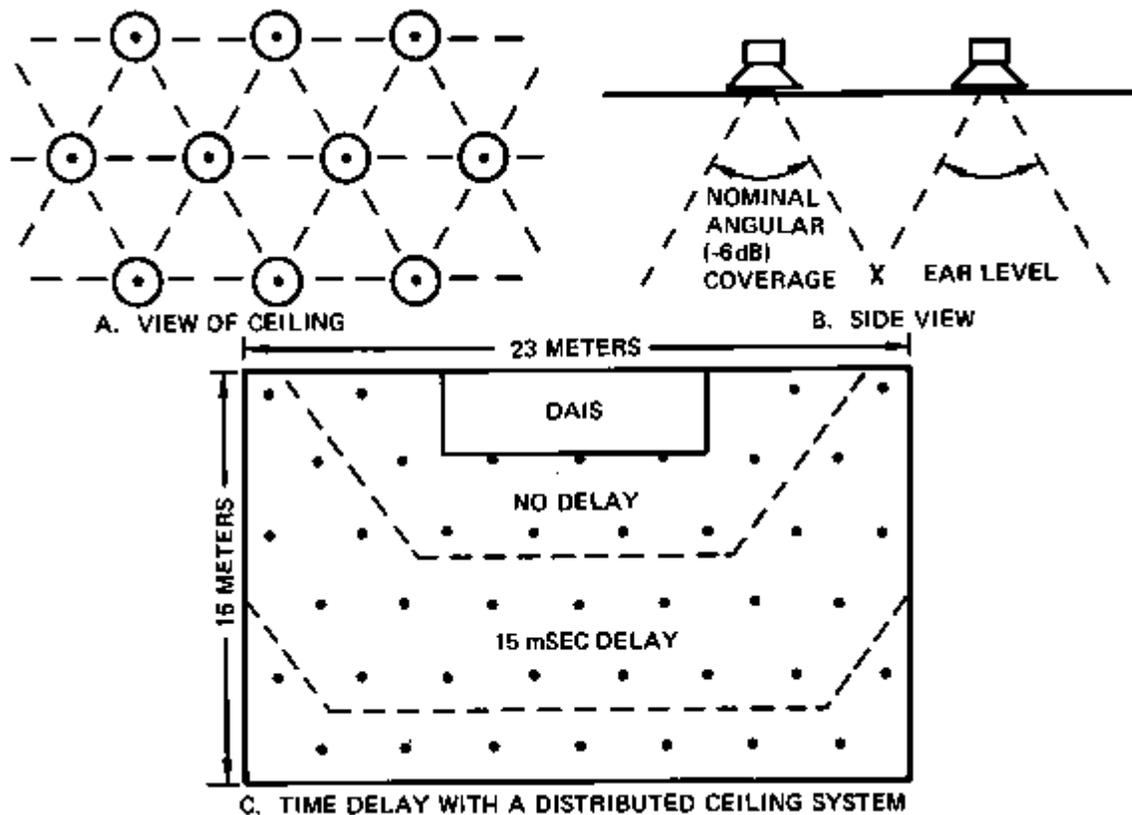
Figure 7-17. Ceiling Lay-out of Distributed Loudspeakers
