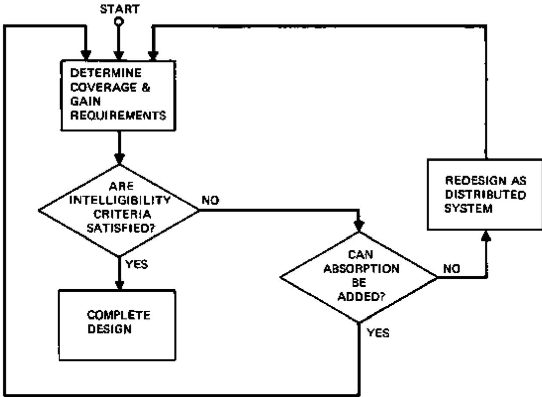
Figure 6-20. Flow Diagram for System Design
