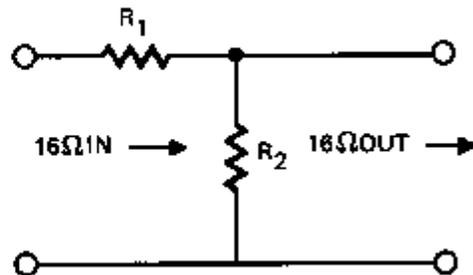
USE ADJUSTABLE WIRE-WOUND RESISTORS OF ADEQUATE POWER RATING.
