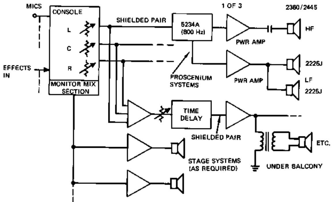
Figure 7-7. A Three-Channel Theater Reinforcement System
