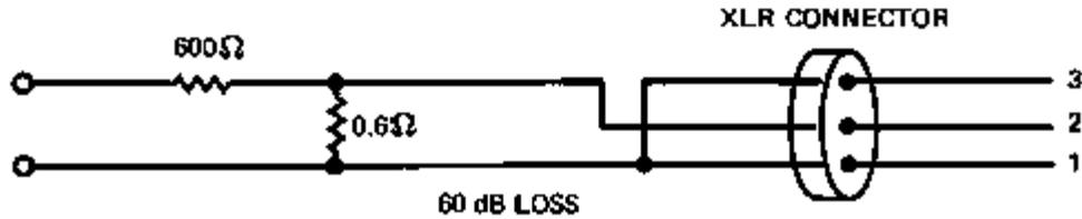
**EXAMPLE: MICROPHONE SENSITIVITY RATING, .0001 volt IN A FIELD OF 74 dB-SPL. SET INPUT TO PAD AT 0.1 volt; OUTPUT IS THEN .0001 volt.**
