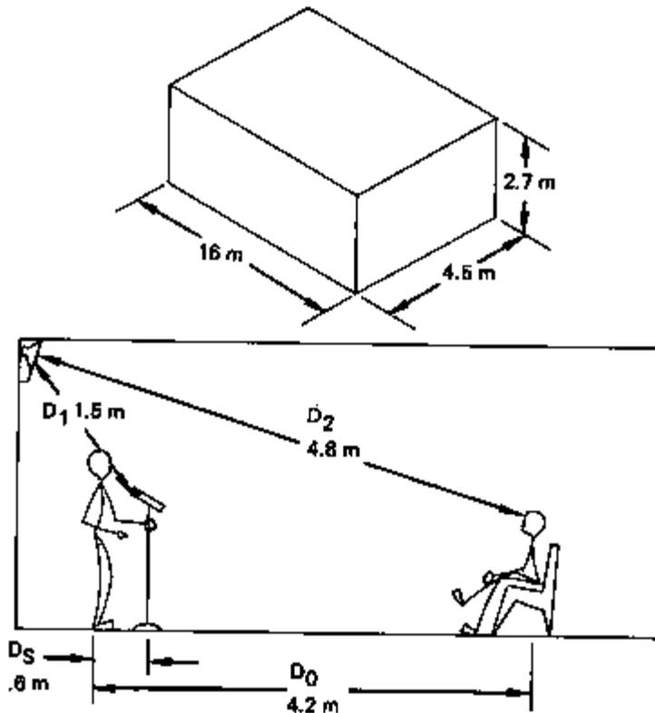
Figure 6-2. Indoor Sound System Gain Calculations
