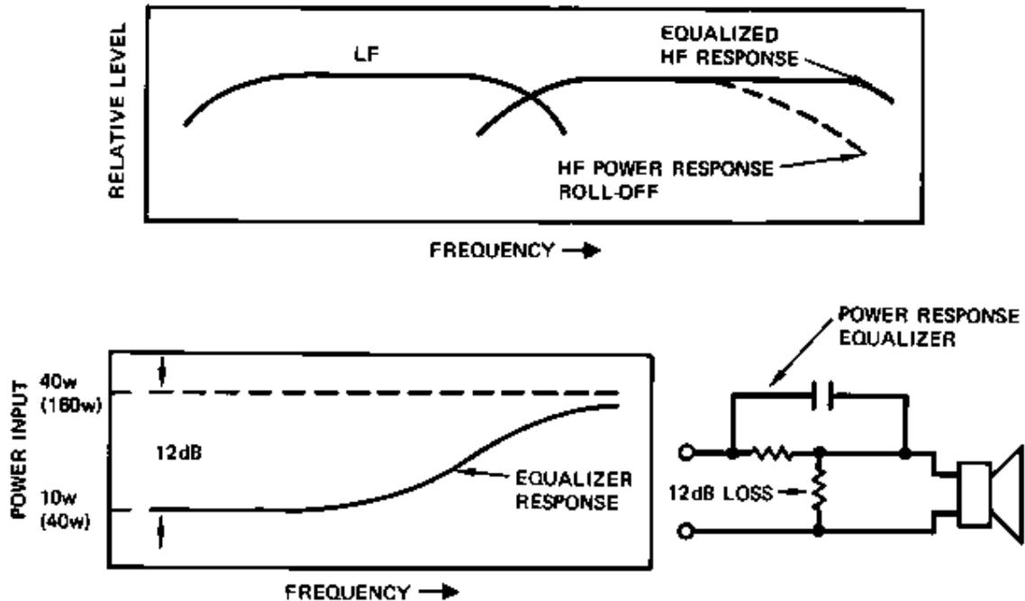
AT MID-FREQUENCIES, HF SECTION CAN BE DRIVEN WITH AS MUCH AS 4 x 40, OR 160 watts;
