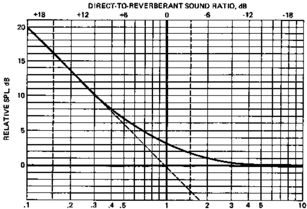
RATIO OF DISTANCE FROM THE SOURCE TO CRITICAL DISTANCE
