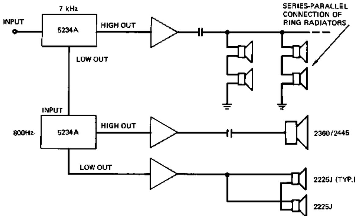
Figure 7-19. HF Augmentation with Ring Radiators
