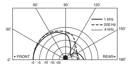
Fig. 3 Horizontal Plane Polar Response
